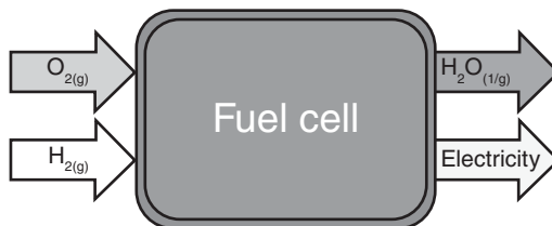
Figure 1.1. General concept of a ( \text{H}_2\text{-O}_2 ) fuel cell.
